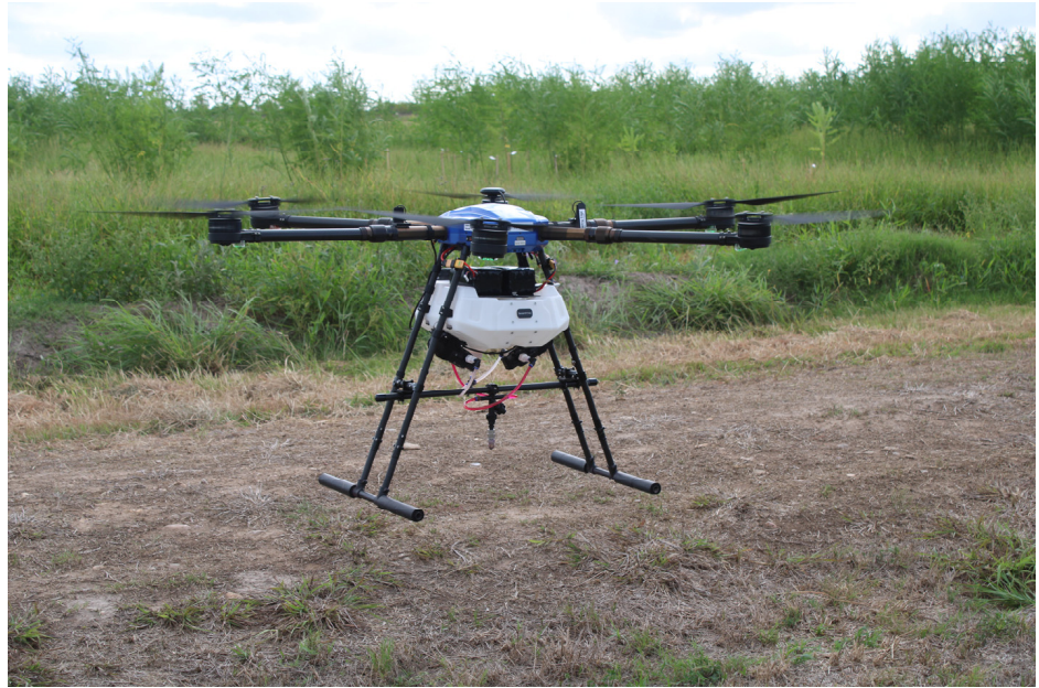
Figure 3. Spray drone outfitted with a conventional spot spray nozzle.
