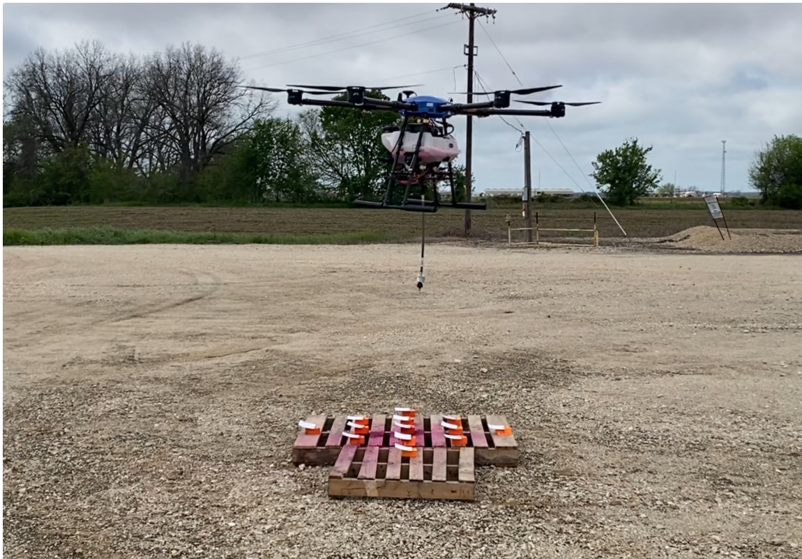
Figure 2. Spray drone outfitted with spot spray drop-nozzle hovering over the center of the targeted area.
