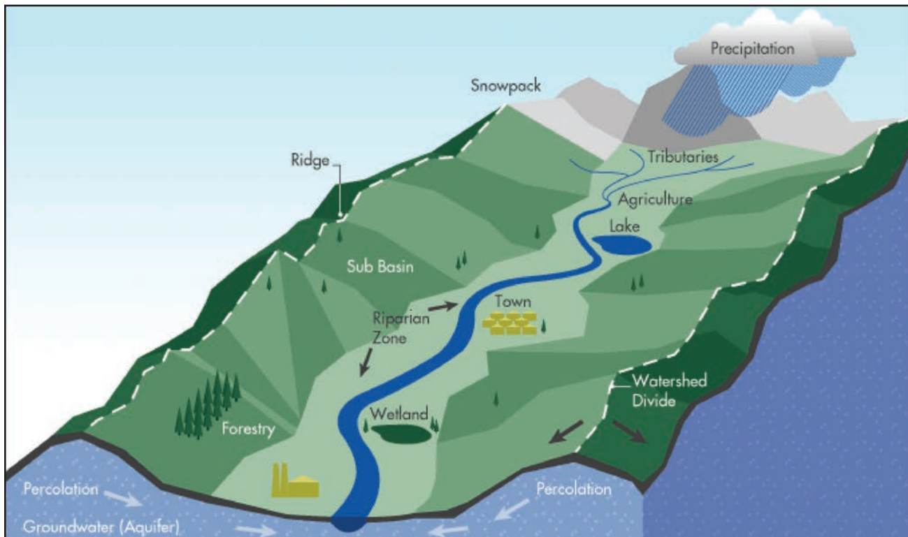
Figure 1. Watershed diagram. (Image courtesy of Pollution Probe: The Source Water Protection Primer, www.pollutionprobe.org/Publications/Primers.html .)
