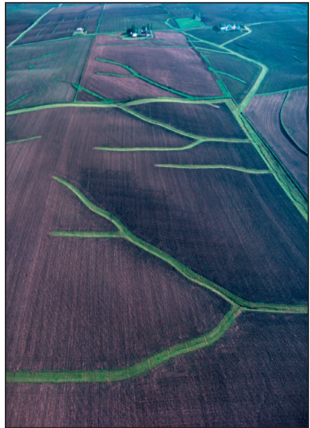
Figure 35. Grassed waterways prevent erosion as they carry runoff from fields. (Photo courtesy of USDA Natural Resources Conservation Service.)
